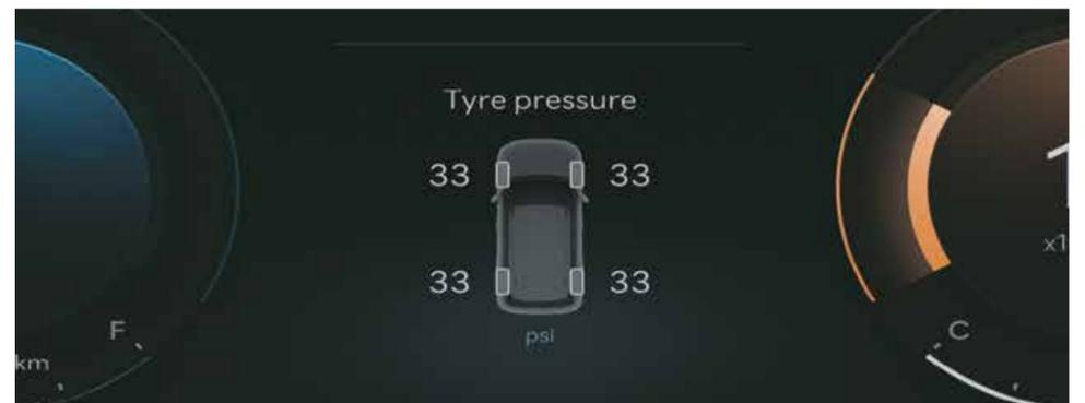
Tyre pressure monitoring system (TPMS) - highline
