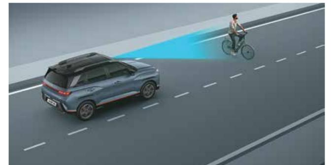
Forward Collision - Avoidance Assist - Cycle (FCA-Cyl)
