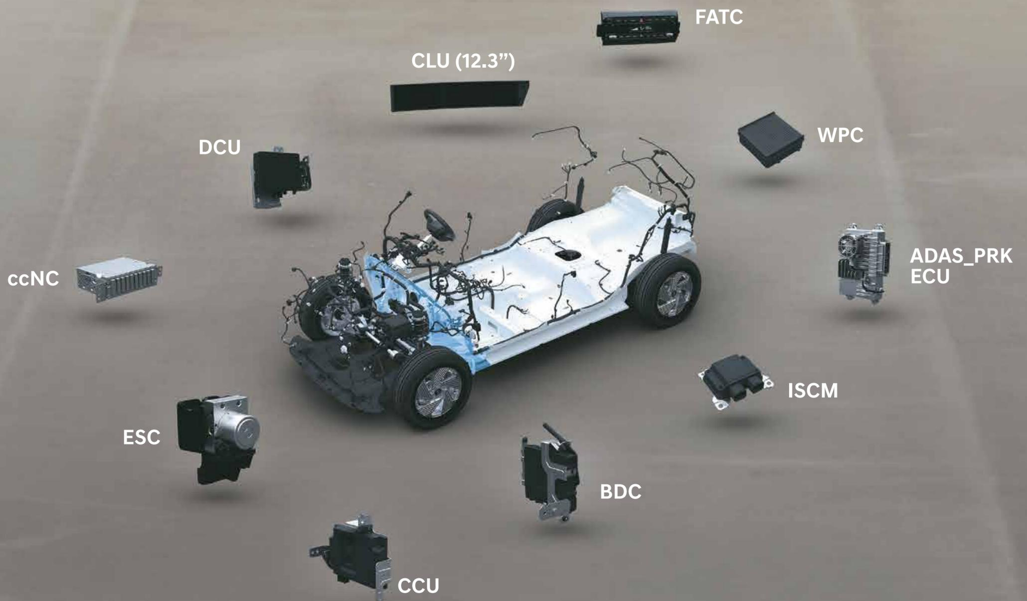
DCU - Data Connectivity Unit | CLU - Cluster | FATC - Fully Automatic Temperature Control | WPC - Wireless Power Charger
