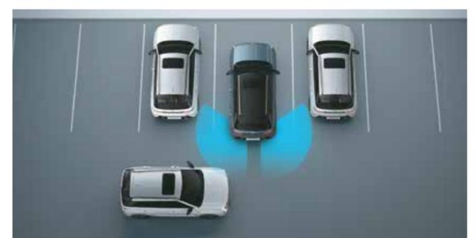
Rear Cross - Traffic Collision - Avoidance Assist (RCCA) & Rear Cross - Traffic Collision Warning (RCCW)
