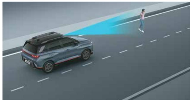
Forward Collision - Avoidance Assist - Pedestrian (FCA-Ped)
